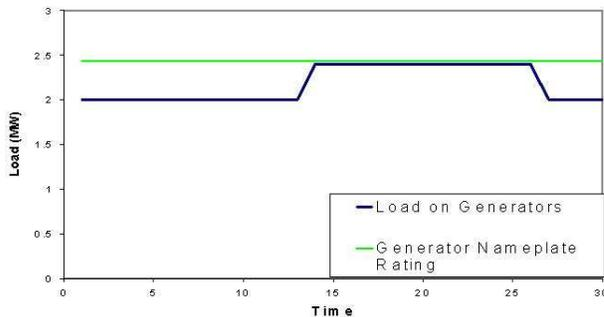
Figure 6: Example Load Profile – 2.5 MW Continuous Rating
