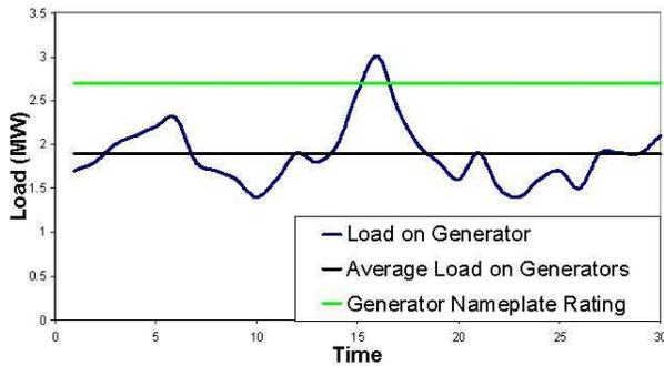
Figure 3: Example Load Profile: 2.7 MW Prime Rating
